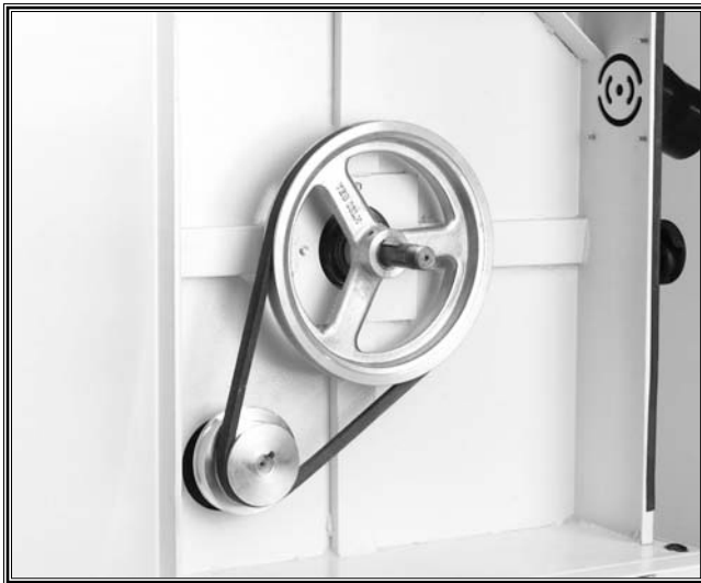
Figure 28. Speed pulley (lower wheel removed for clarity).
